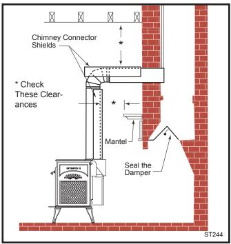
Fig. 6 Chimney connector enters chimney above the fireplace.
